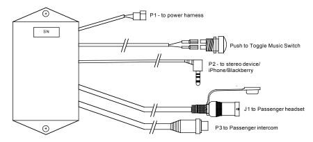
Operation is simple. Press the Push to Toggle switch, and the passenger headset is completely disconnected from the bike's audio system and connected via *MuseSet2*'s internal amplifier to the audio device attached to *MuseSet2*.
