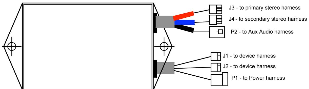
Connect **AuxSwitchSet3** plug, P1 to the Power Harness you installed. Connect this power harness to a *Switched* (*on/off with key*) source.
