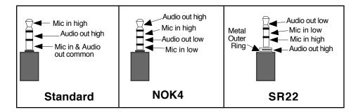
The Standard plug is employed by most cellular telephones, and there are a wide array of adapters available that allow this plug to connect to phones with proprietary or differently wired headset jacks via an adapter.
